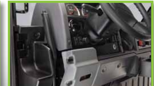
The brake fluid reservoir has an access panel with a viewing window. The park brake is left of the driver's controls.
