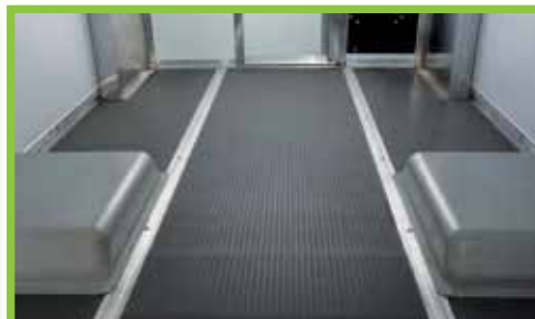
Composite floor with slip-resistant vinyl floor overlay.
